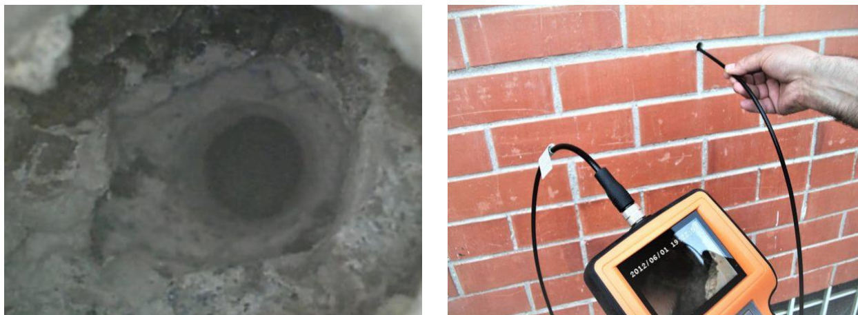
Figure 71: Execution of endoscopic test
