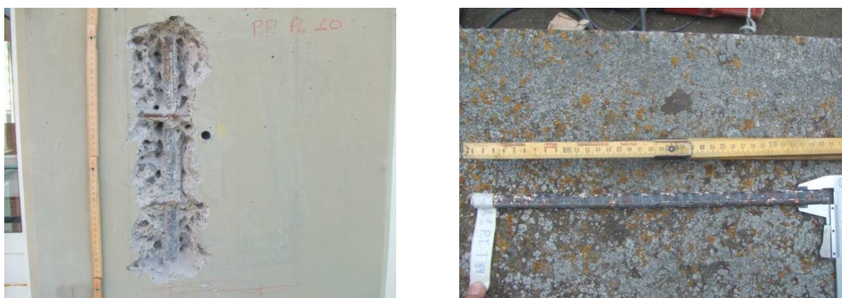
Figure 66: Extraction of steel bars and steel sample.
