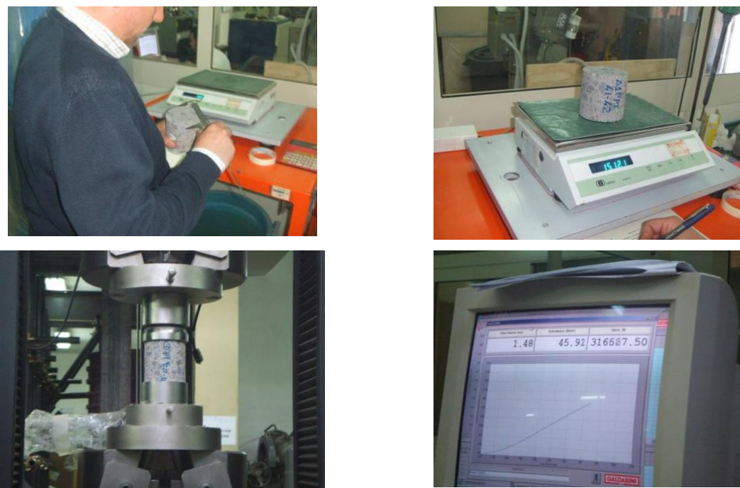
Figure 70 Execution of uniaxial compression test.
