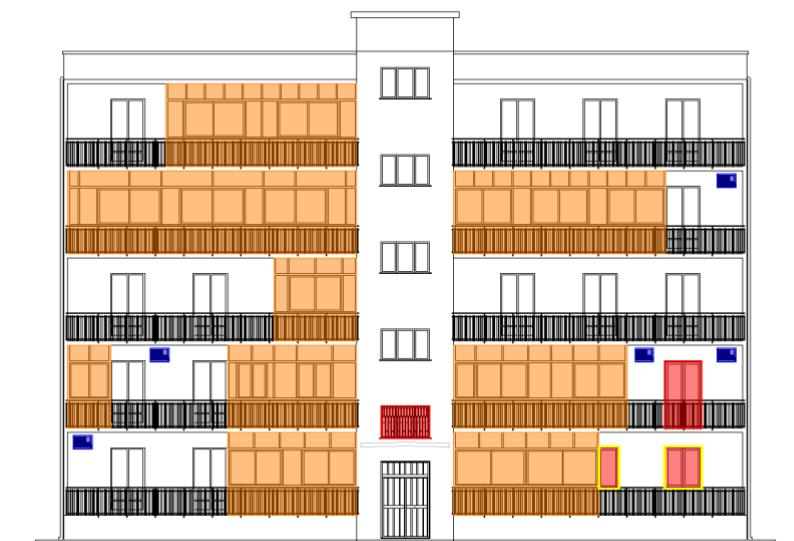
Figure 18: South elevation with the transformations by the residents. The “verandas” are shown in orange. The demolitions of the interior walls are shown in red. The air conditioners are shown in blue.
